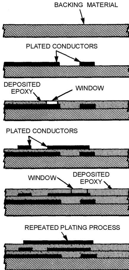
Figure 1-42.—Layer build-up technique.
