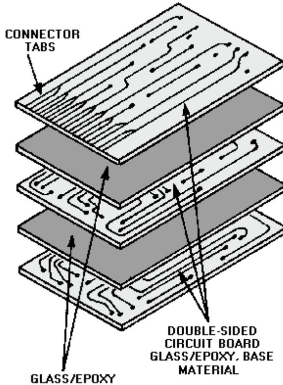
Figure 1-39.—Multilayer pcb.
