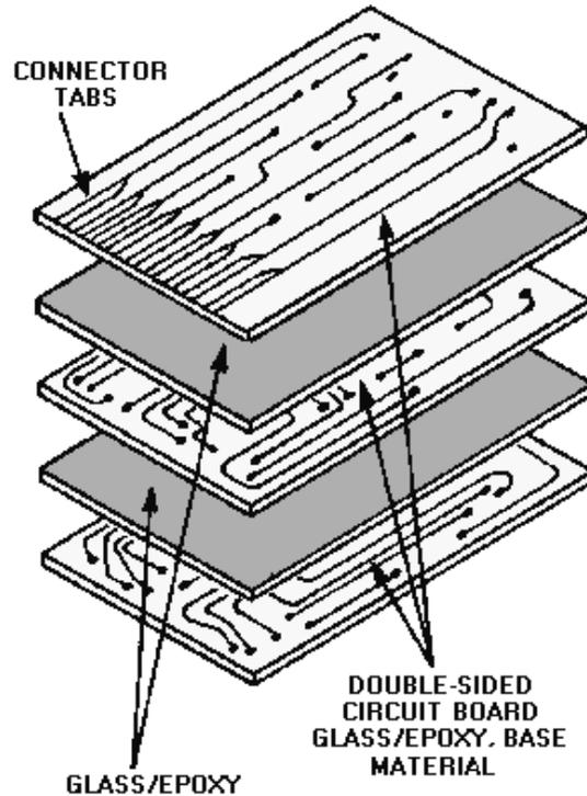
Three methods of interconnecting circuitry in multilayer printed circuit boards are the **CLEARANCE-HOLE**, the **PLATED-THROUGH-HOLE**, and **LAYER BUILD-UP**.
