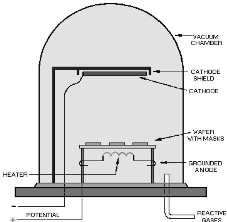
Figure 1-16.—Cathode-sputtering system.
