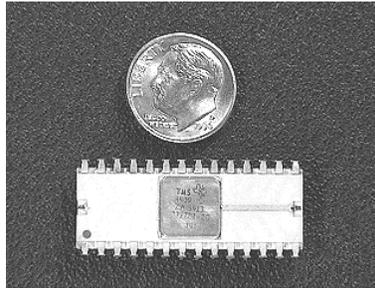
Figure 1-25.—Dual inline package (DIP).
