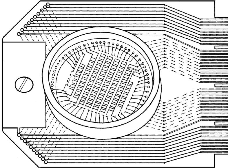
**Figure 1-6.—Large-scale integration device (lsi).**
