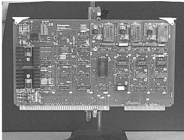
A **MICROCIRCUIT MODULE** is an assembly of microcircuits or a combination of microcircuits and discrete components packaged as a replaceable unit.
