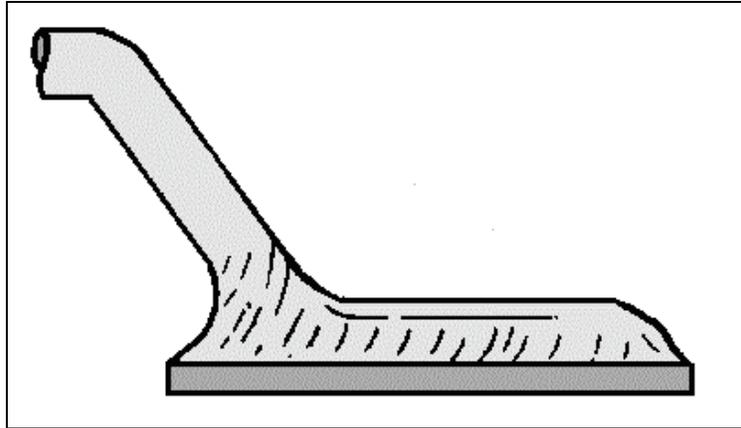
Figure 3-9.—On-the-board termination.
