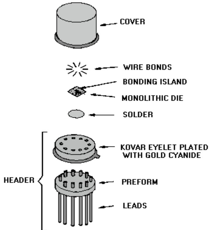
Figure 1-19.—Exploded TO-5.
