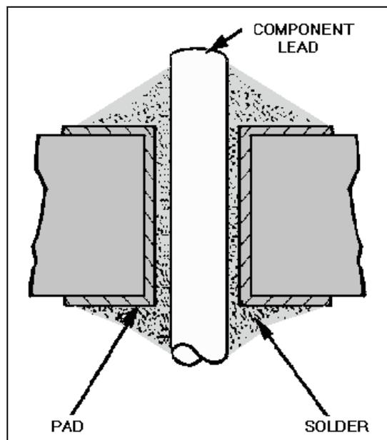
Figure 3-6.—Straight-through termination.
