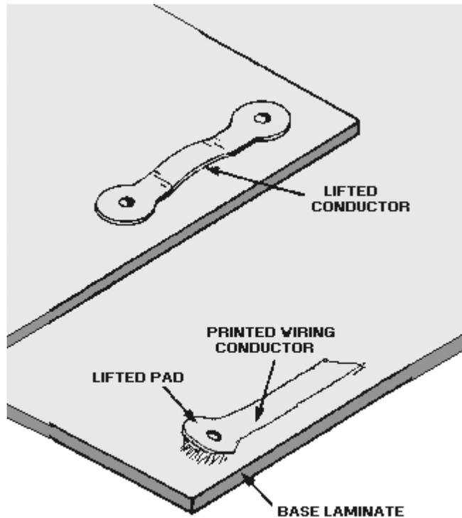
Figure 3-26.—Delaminated conductors.
