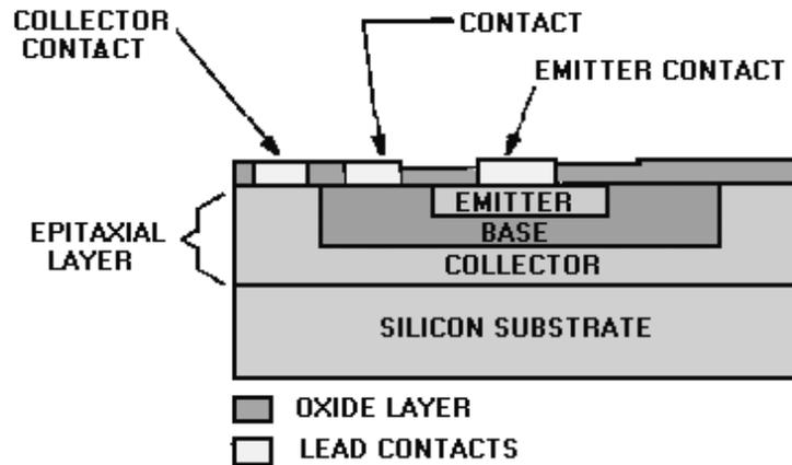
Figure 1-13.—Planar-epitaxial transistor.
