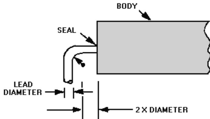
Figure 3-13.—Minimum distance lead bend to component body.
