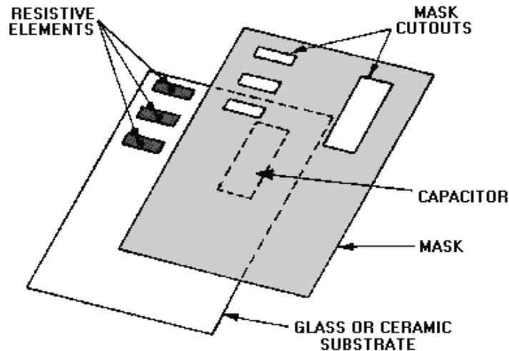
Figure 1-17.—Cathode-sputtering mask.
