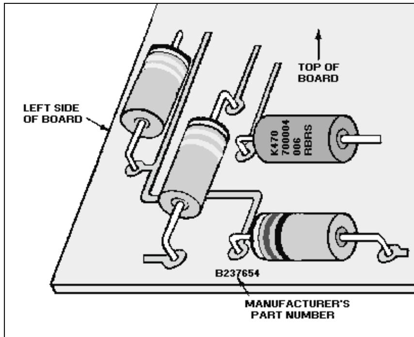
Figure 3-15.—Component arrangement.
