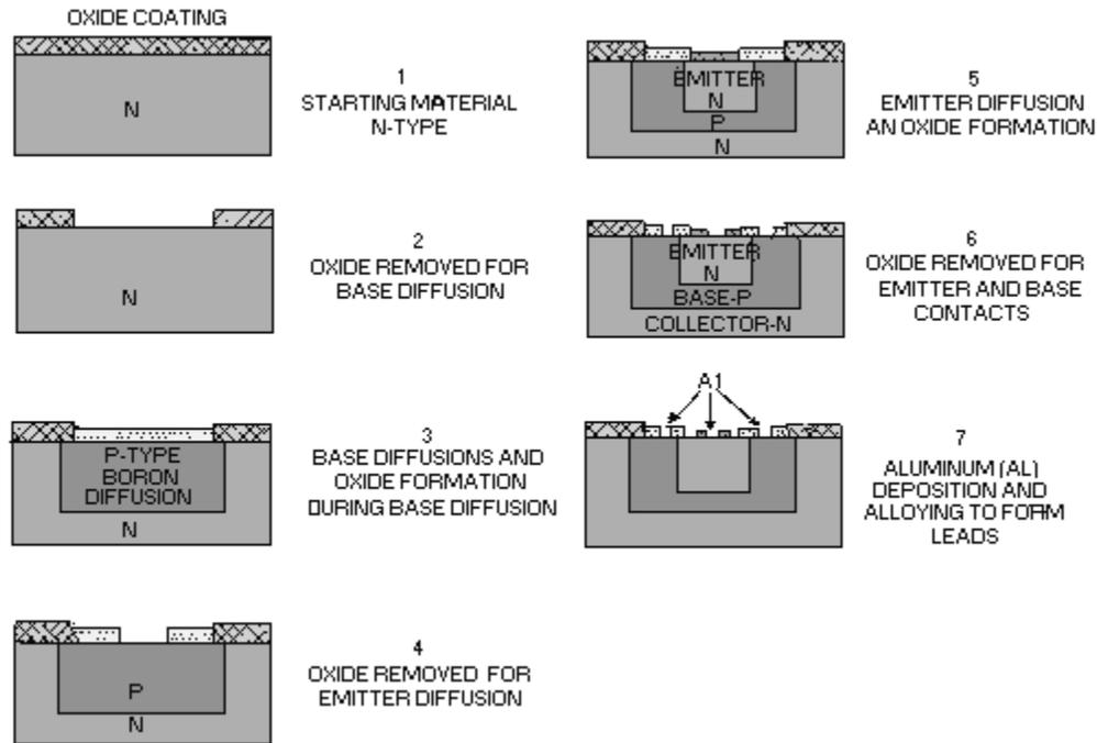
Figure 1-12.—Planar-diffused transistor.
