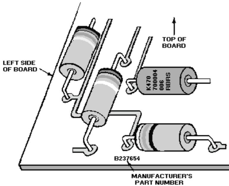
A **GOOD SOLDER JOINT** is bright and shiny with no cracks or pits.
