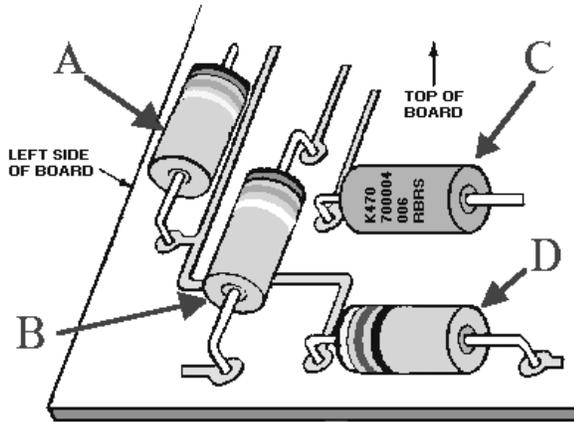
Figure 2A.—Component mounting.
