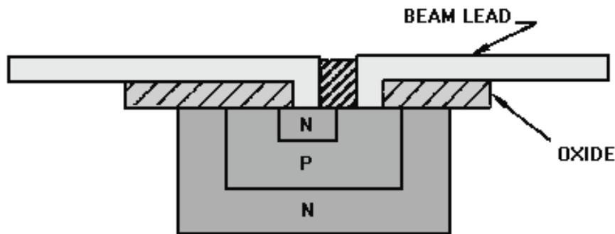
Figure 1-27.—Beam-lead technique.
