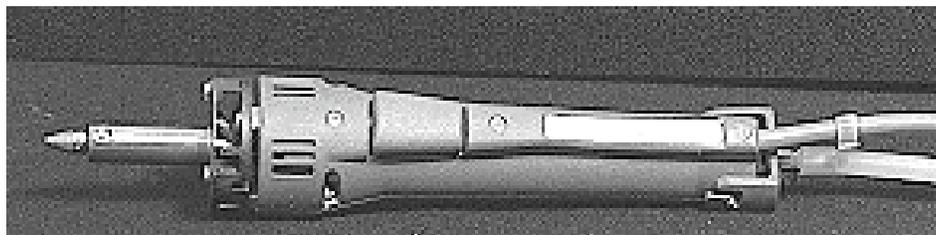
**Figure 2-3.—Motorized solder extractor.**
