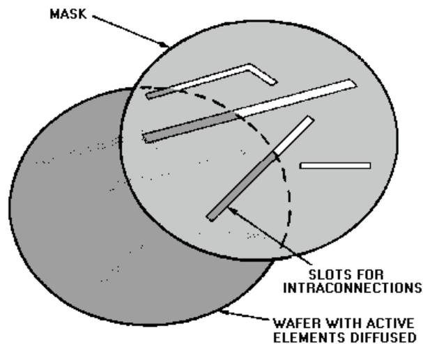
**Figure 1-15.—Evaporation mask.**
