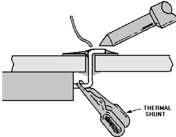
Figure 3-16.—Thermal shunt.
