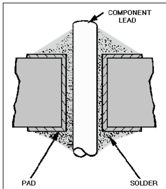
Figure 3-6.—Straight-through termination.
