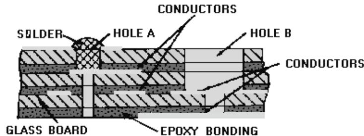
Figure 1-40.—Clearance-hole interconnection.
