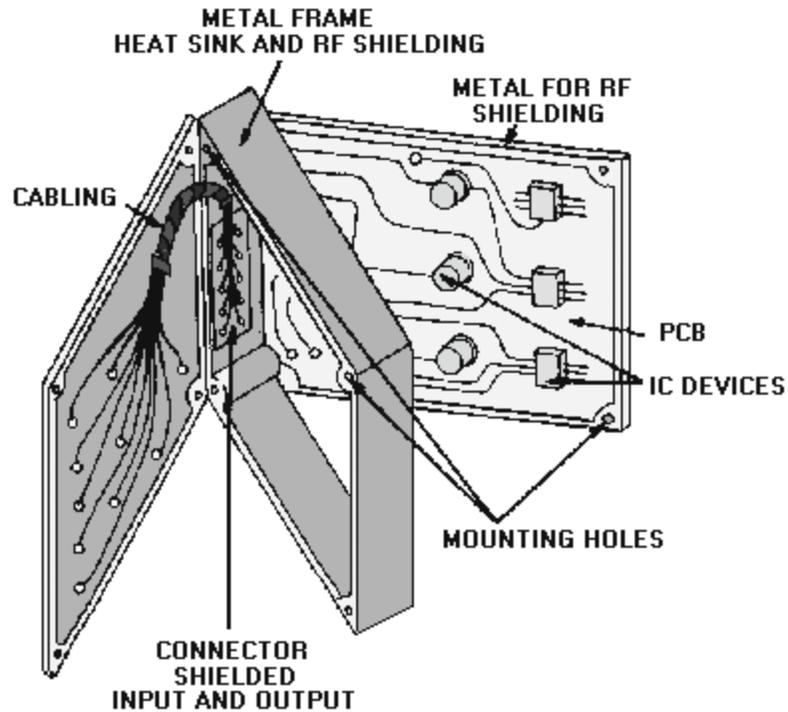
Figure 1-44.—Ground planes and shielding.
