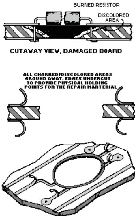
Figure 3-29.—Repair of burned boards.
