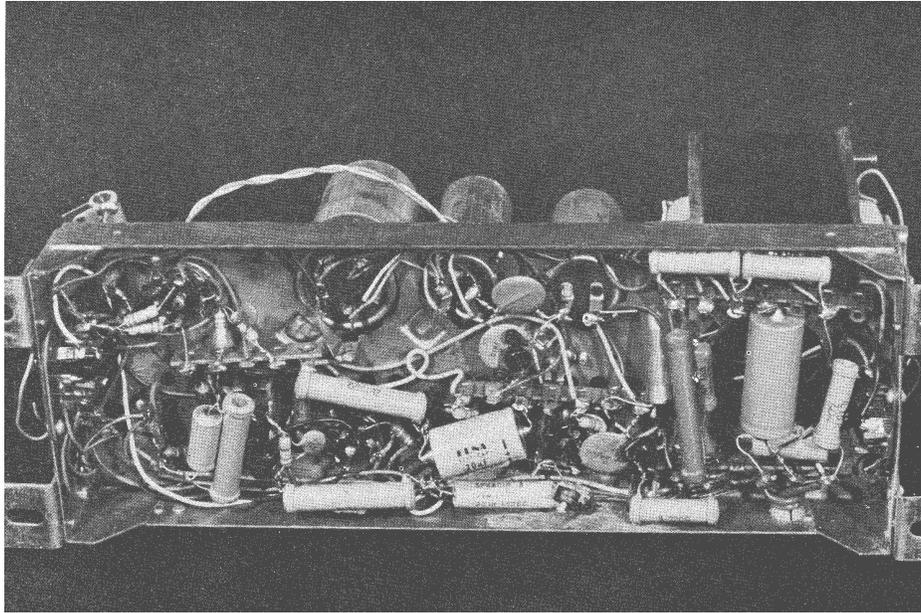
**Figure 1-2.—Point-to-point wiring.**
