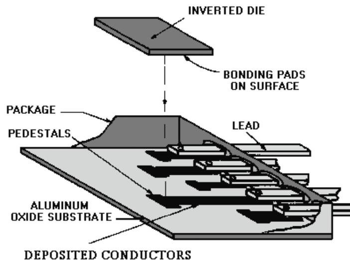
Figure 1-26.—Flip-chip package.
