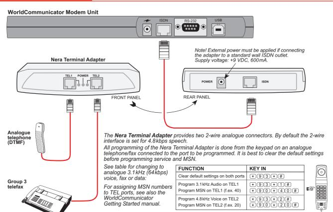
The adapter is powered via the ISDN connector when used with the WorldCommunicator. No external power is then required.
