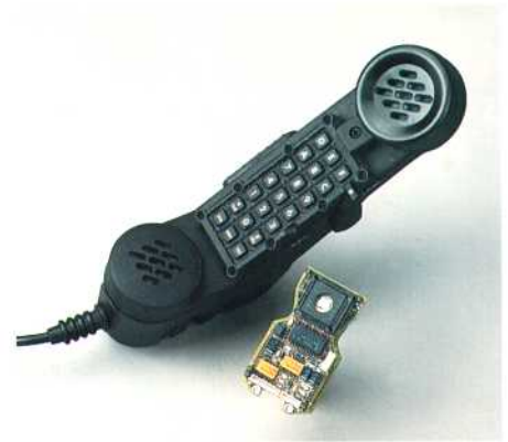
The DSP 9000 handset replaces the radio handset for manpack applications.
