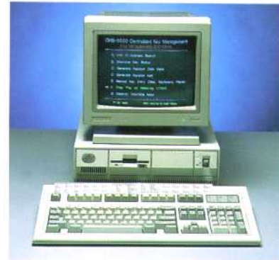
The crypto management system facilitates key generation, loading, and distribution.
